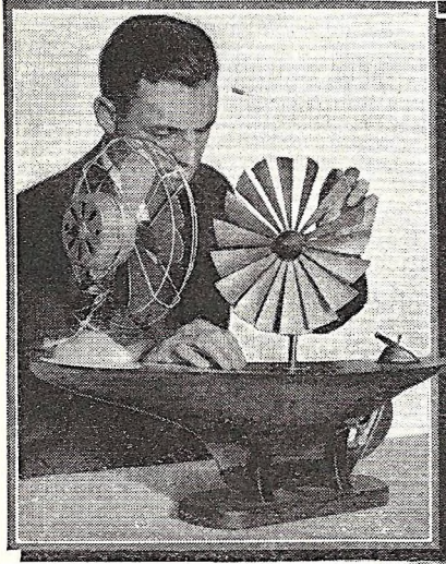
Air blast from fan turns windmill mounted on model boat, in demonstration at English inventor's exhibit. At right is artist's conception of ocean liner using the wind-propeller sails.
