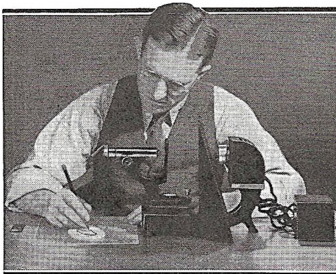
Mirror clipped to eyepiece tube throws image of specimen onto paper where it may be easily and accurately traced.
