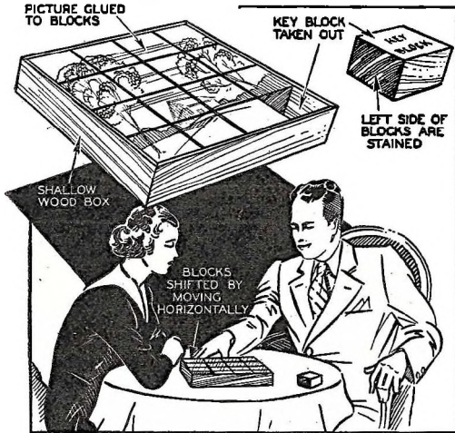
In novel variation of 15 block puzzle, picture glued to blocks is scrambled, then blocks shifted to form it again. Stain one side of blocks to facilitate replacing in box.
