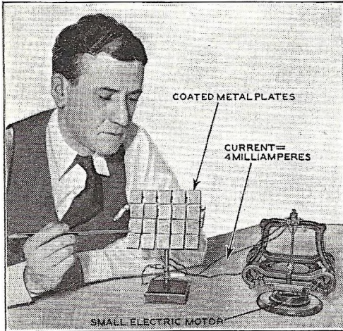
J. Thomas Rhamstine points out photo-electric plates used in his miniature solar power plant. Sun's rays striking the 20 squares generate current of 4 milliamperes, enough to run the midget electric motor shown at right. Oxide coating on face of metal plate converts light to electricity.
