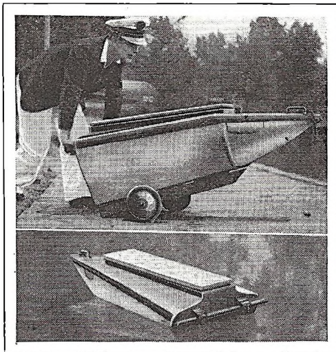
Top photo shows carriage for launching the rescue craft. Below—Device in the water. Note the towing handles.
