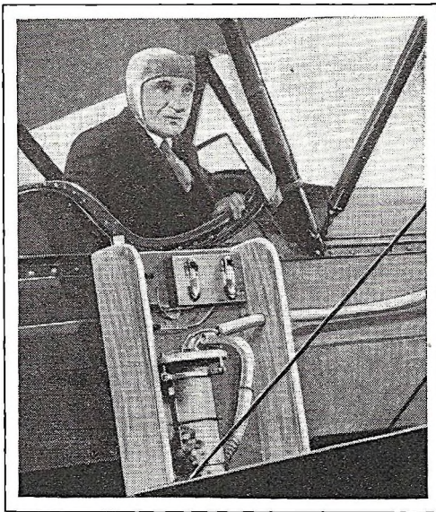
A closeup of the air-collecting device is shown attached to side of cockpit. Specimens are taken at various heights.
