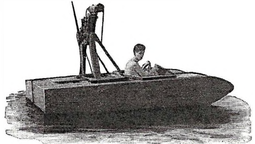
Gordon Lyons built this hydroglider. It is powered with a twin cylinder motorcycle engine. It travels fifteen m. p. h.
