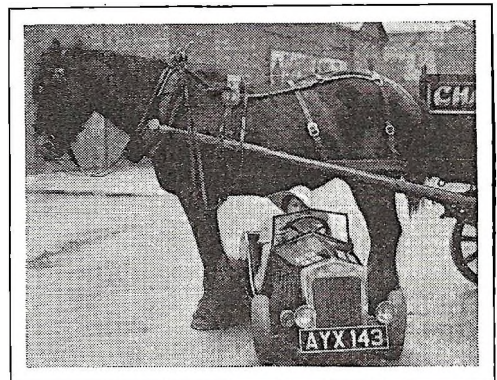
Now in quantity production in England, this midget car averages about 15 m.p.h. and travels 70 miles to the gallon.
