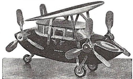
A cam-and-shaft arrangement in propeller hubs enables blades to be tilted at will of pilot. When striking air flat, blades are said to effect vertical climb or descent.
